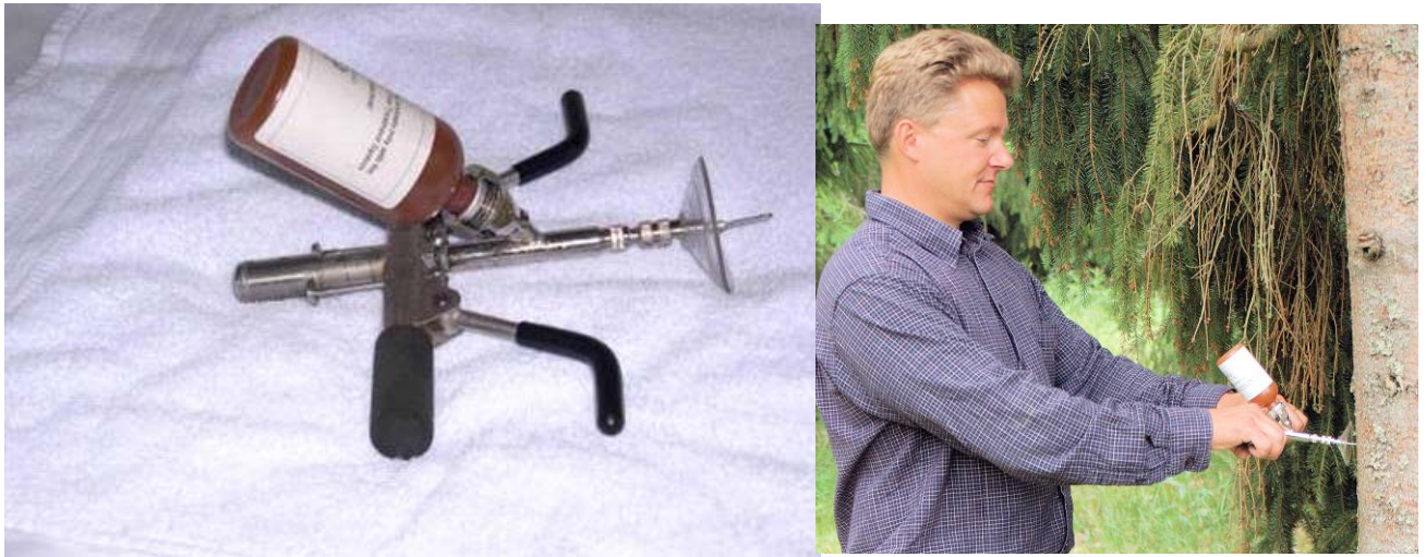
Figure 2. The Wedgle™ Direct-Inject™ tree injection unit from ArborSystems (Omaha, USA) tested in 504 Ålbrunna.
